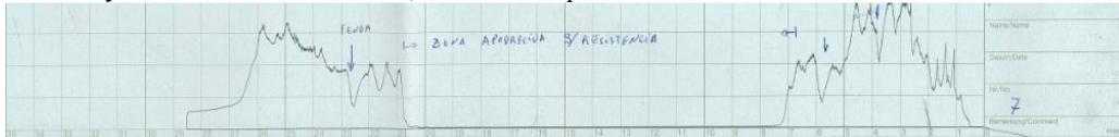
Fig. 6. Obtained graphic of the R4 beam of the pavement, through resistograph (image from: [9]).
