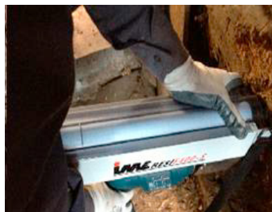
Fig. 1. Resistograph used in this study (images from: [9]).
