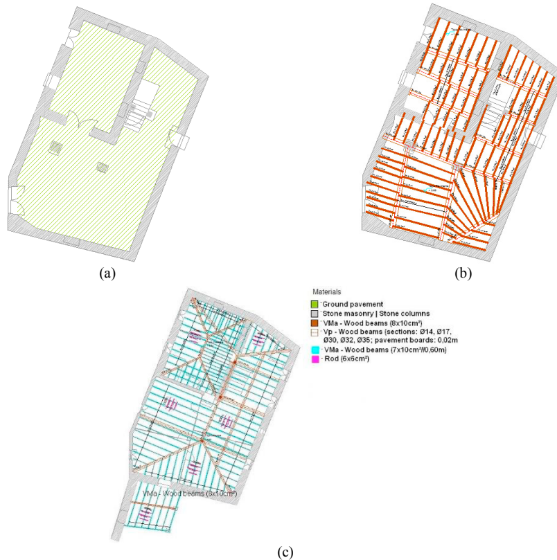
Fig. 3. Structural plants: (a) basement; (b) first floor; (c) roof (images adapted from: [7]).
