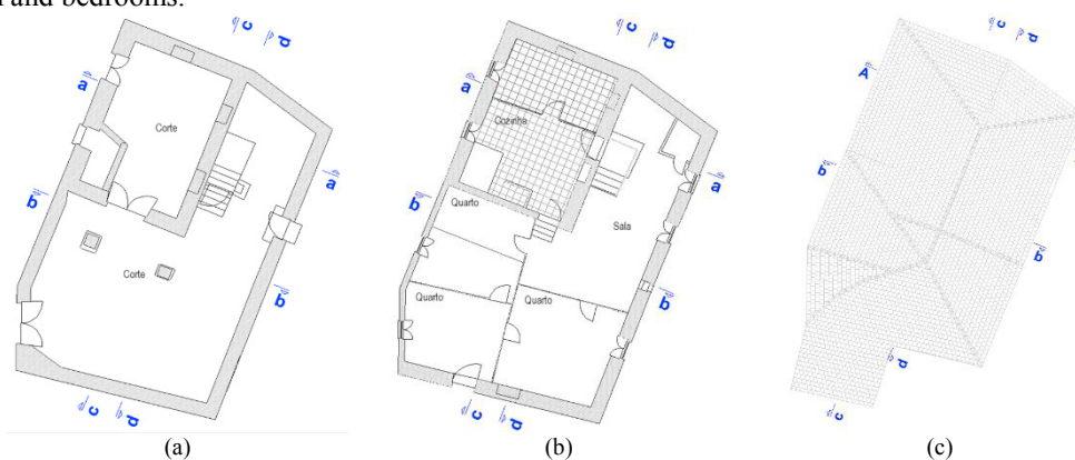
Fig. 1. Architectural survey of the building: (a) basement plant; (b) first floor plant; (c) roof plant (Images from: [7]).
